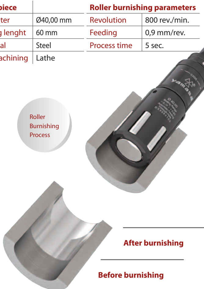
Figure 3 - Before and after roller burnishing surfaces
